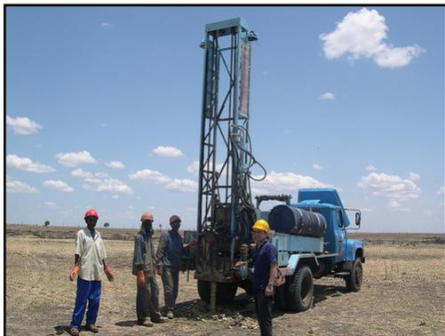
On land seismic operations involve the generation of seismic vibrations by explosive or mechanical sources. One type of energy source for seismic exploration is an explosive charge. Small holes ("shot-holes"), typically 4 inches in diameter, are drilled into the earth surface 10'-60' deep depending on surface terrain,<sup>3</sup> although some drill holes have been drilled to 200'.<sup>4</sup> The photo to the left shows an example of a shot-hole drill unit.
