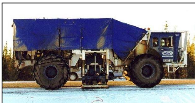
The use of thumper trucks is not considered best practice because it involves dropping a steel slab that weighs about three tons to the ground to create a seismic vibration. Thumper trucks are large, requiring extensive tree and vegetation removal, and leave land scars.
